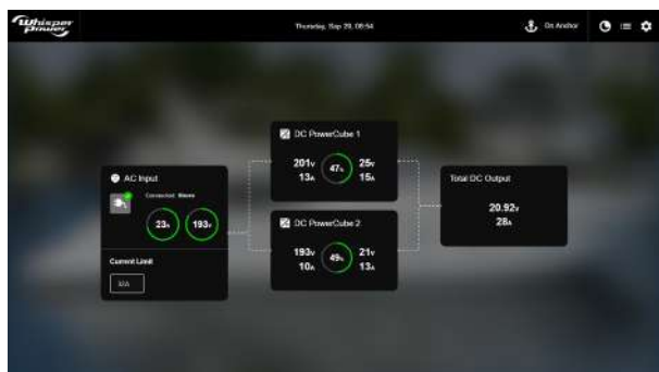
Summarized input and output power data combined from all chargers in a system
