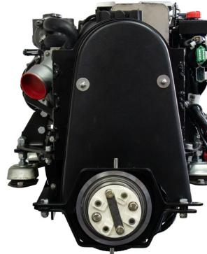
This parallel hybrid system can be fitted to a vessel during its initial construction. The hybrid system does not disturb the normal shaft / propeller connection to the diesel, instead as the name implies it connects to the shaft in parallel with the standard diesel engine. Hybrid systems have the most to offer inefficiency improvements during low to mid power cruising
