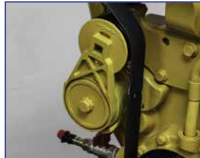
Automatic spring loaded belt tensioner
