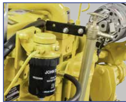
Lube oil drain pump
