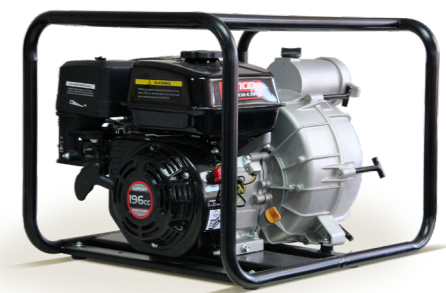
LC80WB30-4.5Q5 SEMI TRASH PUMP - 3" discharge diameter - 30 metre lift - 45,000 litre delivery volume - 39 kg net weight
